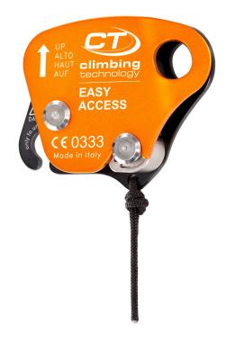
Fall arrest device specifically designed for use in rope access work, compliant with the standard EN 12841-A. It has been designed to remain constantly positioned above the user, thus minimizing the potential fall factor to the minimum.
