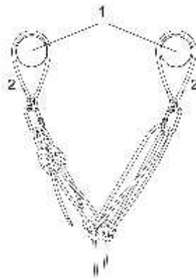
b) Example of double protection being provided by the use of eyebolts
